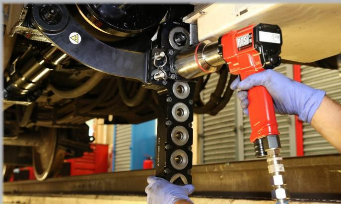
Lower bolt using long reaction
