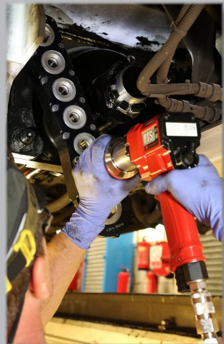
Upper bolt using one of the short reaction orientations
